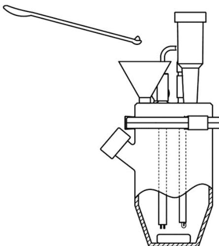
Fig.3.3 Introduction of sample with powder funnel
