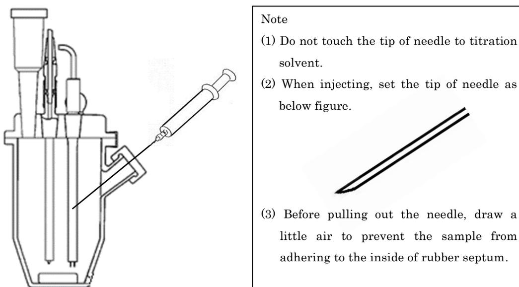
Fig.3.2 Injection of sample
