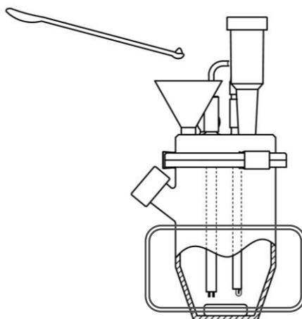
Fig.3.4 Introduction of sample with powder funnel
