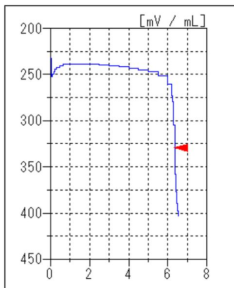
Measurement for total sodium chloride
