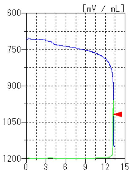
Titration curve for hydrogen peroxide
