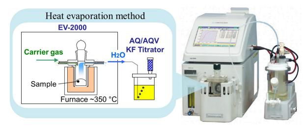
Fig.3.3. Schematic diagram of heat evaporation method.
