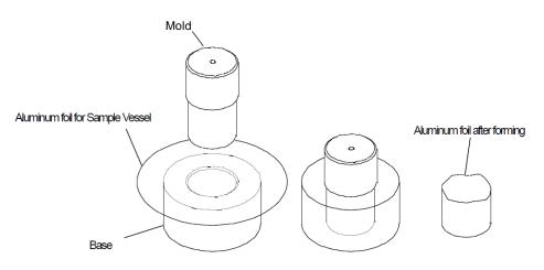
Fig.3.2. Forming the aluminum foil.
