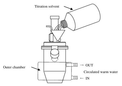
Fig.3.1 Preparation of the reagents
