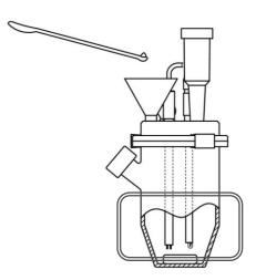
Fig.3.4 Introduction of sample with powder funnel
