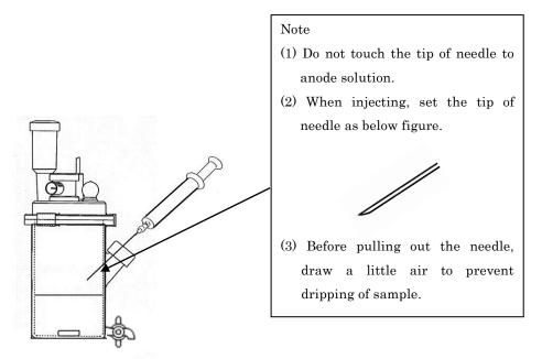
Fig.3.2. Injection of sample.
