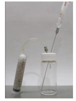
Fig.5.1. Draw the sample from syringe vial.
