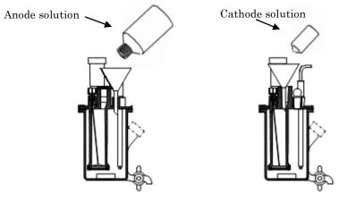
Fig.3.1. Preparation of the reagents.
